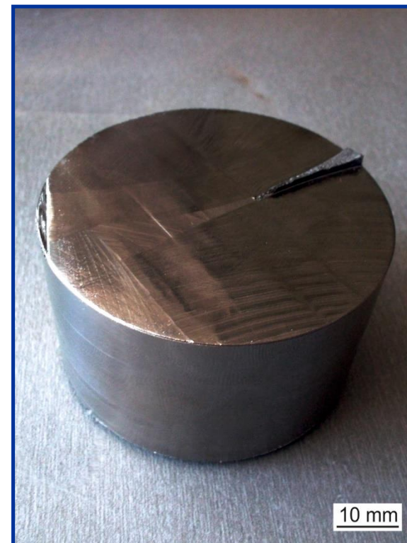
Initial ingot subjected to HIP-ing at 1280 °C for 4 h at 200 MPa.
