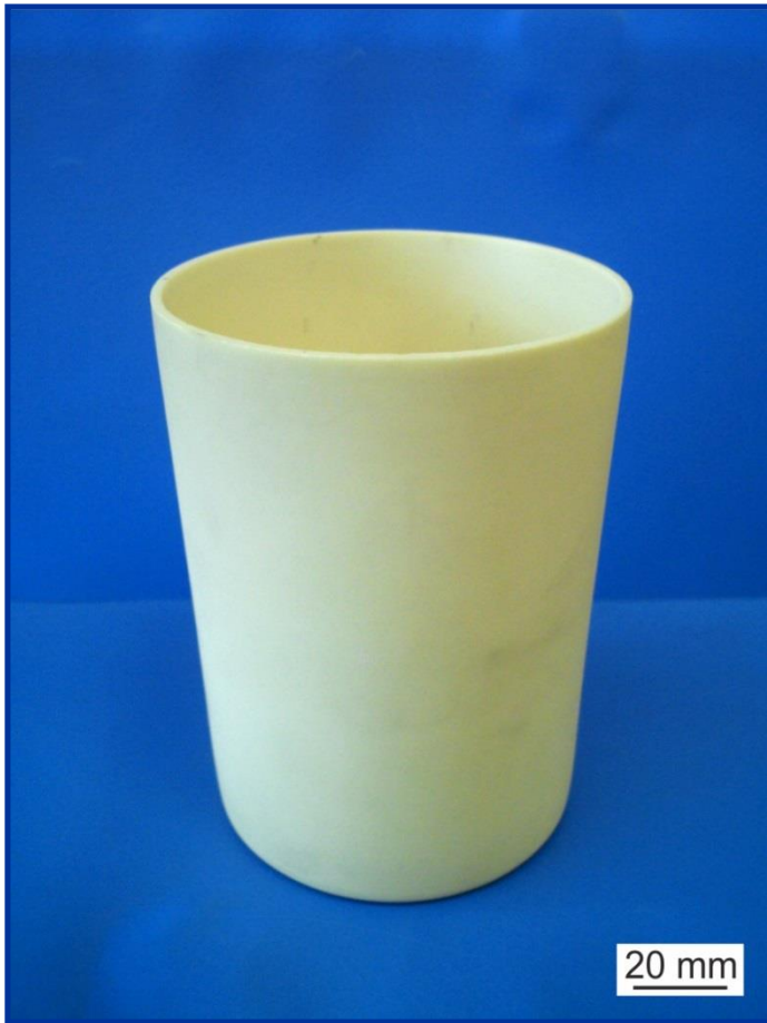
Pure Y_2O_3 crucible for induction melting.
