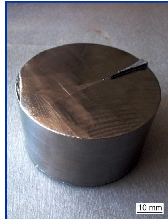
Initial ingot subjected to HIP-ing at 1280 °C for 4 h at 200 MPa.
