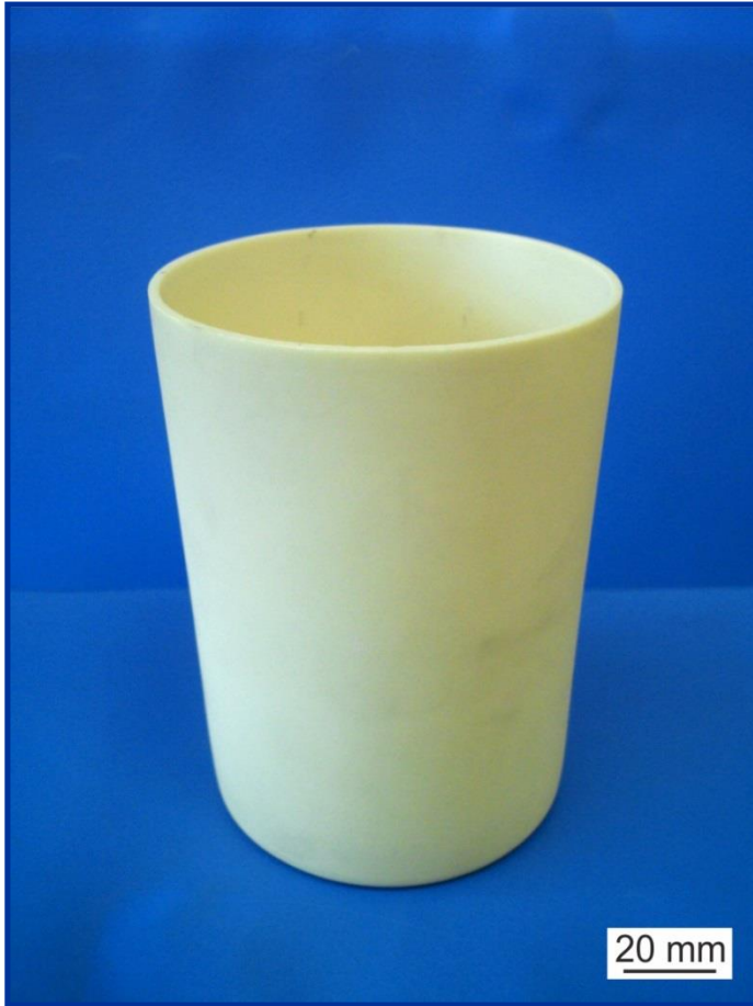
Pure Y_2O_3 crucible for induction melting.
