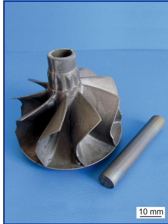
Extracted sample for mechanical testing from as-cast turbocharger wheel.
