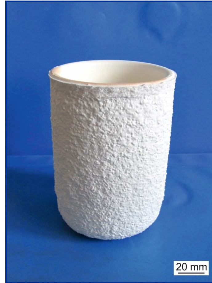
Al_2O_3 based crucible with inner Y_2O_3 layer for induction melting.
