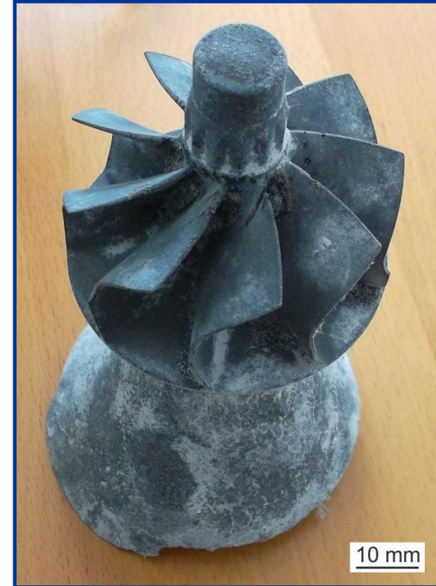
Rough casting removed from the mould.
