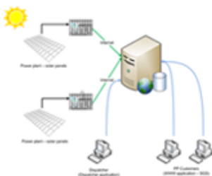
POWER PLANT MONITORING SYSTEM - PPMS
